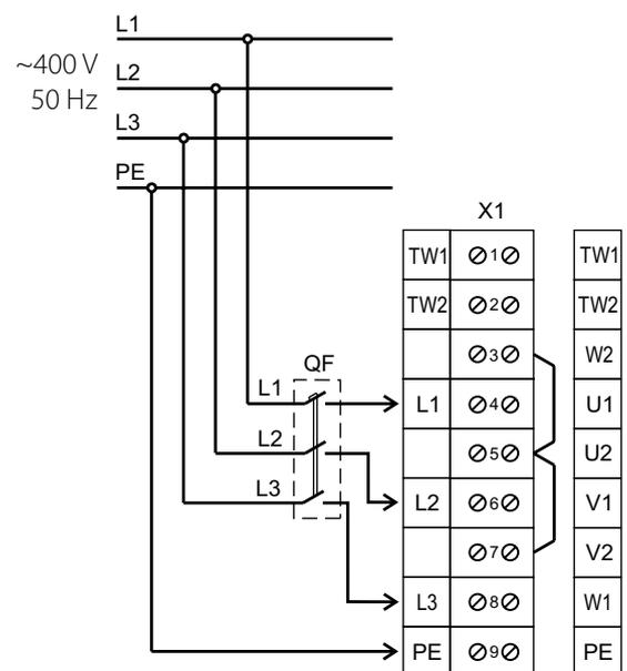
\* X1 – terminal block, QF – automatic circuit breaker (not included in the delivery set).
